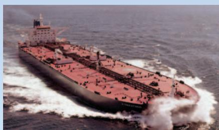
**Tankers** transport crude oil, chemicals and petroleum products. More than 70% of the world's ocean going tankers now have double hulls.
