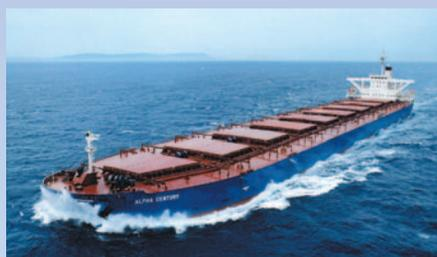
**Bulk Carriers** are the work horses of the fleet, transporting raw materials such as iron ore, coal and foodstuffs, and are identifiable by the hatches raised above deck level which cover the large cargo holds.
