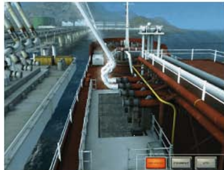
Kongsberg LPG carrier manifold simulation, showing frosted loading arms
